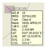
Each target is identified with the ship's name if it is known. When the name is empty or is '?' in the ship list, the MMSI is shown instead.
