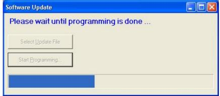
• When the file has been fully sent to the easyTRX, the device must re-boot again. Newer software does this automatically. When you see this message, wait a few seconds and then turn the power off and back on after some more seconds. Do not disconnect the serial connection to the PC.
