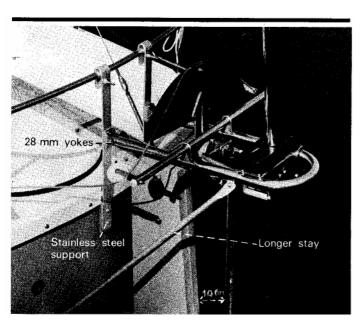
Remember, the mounting bracket must always be 80/90 cm (32/36") above the waterline and the paddle and shaft at least 10 cm (4") behind the rudder.
