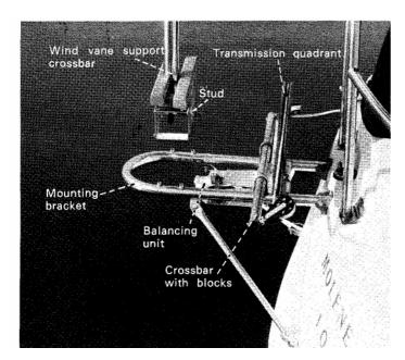
Now, carefully position the wind vane support crossbar onto the rear of the mounting bracket taking care to engage the stainless steel stud on the crossbar into the black nylon bearing at the rear of the cast alloy balancing unit. Tighten the four 6 X 10 mm bolts which hold the crossbar unit to the mounting bracket.
