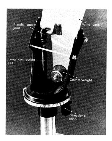
Lock the wind vane. The stainless steel ba.ll-link at the lower part of the wind vane support must be in a vertical position.
